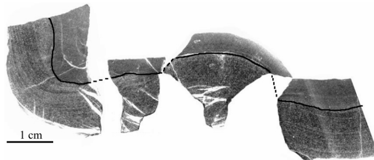
Fig. 6. Scanned image of the hinges of fold A, with curvature related to dissolution seams (stylolites) 'removed'. See text for discussion.
