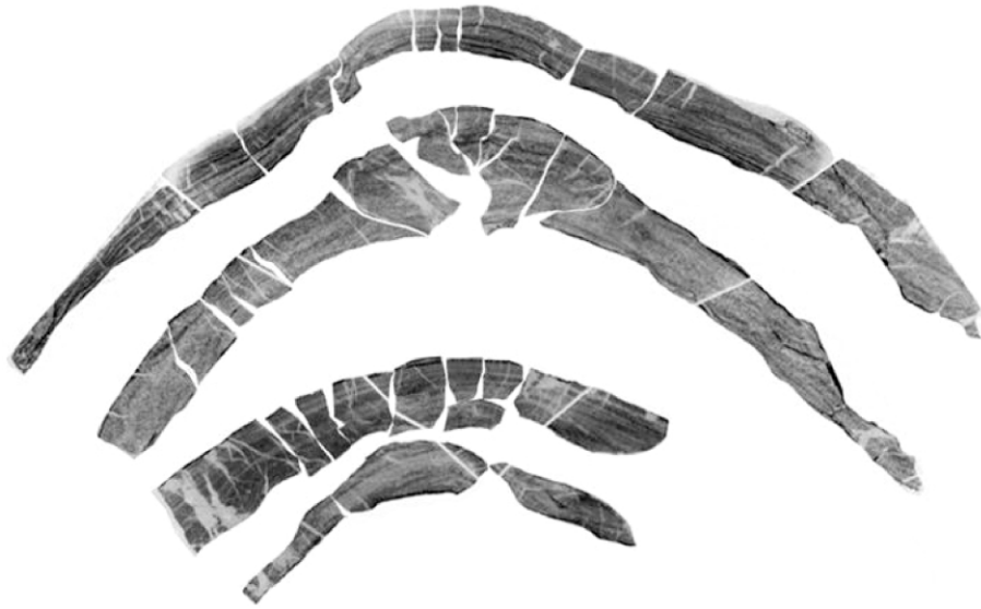
Fig. 10. Four 'layers' of fold B, with curvature accommodated by veining graphically 'removed'. Compare with Fig. 5b. Note that bed-normal veins accommodate a significant amount of curvature, but certainly not all of it.
